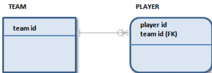
Standard IE notation does not include rounded corners on entities. Rounded entity corners are an IDEF1X symbol included in IE notation to help ensure compatibility between methods.
