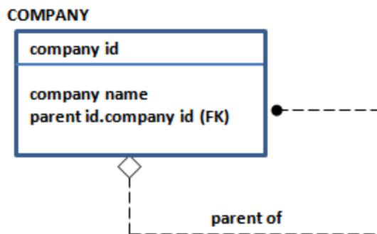
The recursive relationship for COMPANY includes the diamond symbol to indicate that the foreign key can be NULL, such as when a COMPANY has no parent. Recursive relationships must be both optional (diamond) and non-identifying.
