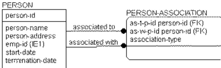
However, the DBMS schema function does not support a data type of *list*. Since the schema is a representation of the database in a physical relational system, first normal form errors are also prevented at this level.
