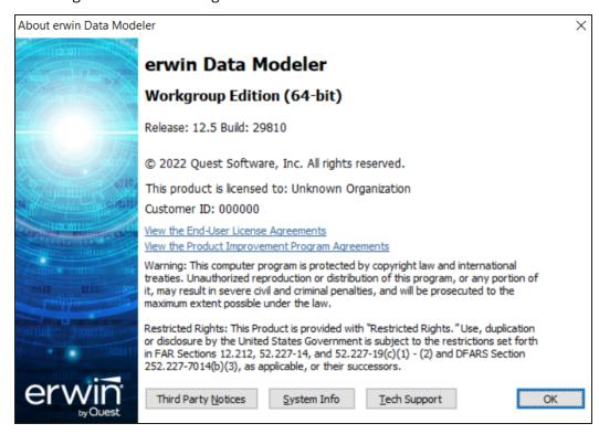
Release indicates the main (GA) release number and the second number (if available) indicates the patch or service pack number of the main release. Build indicates the build number of the product. For example, "Release: 12.5 Build: 29810" on the above screen indicates Release 12, Patch 5, Build 29810.
